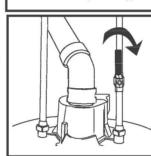
water to the water heater. Note that the top of the water heater will usually be marked "Cold" or "Inlet" at the point where the cold water line is connected
